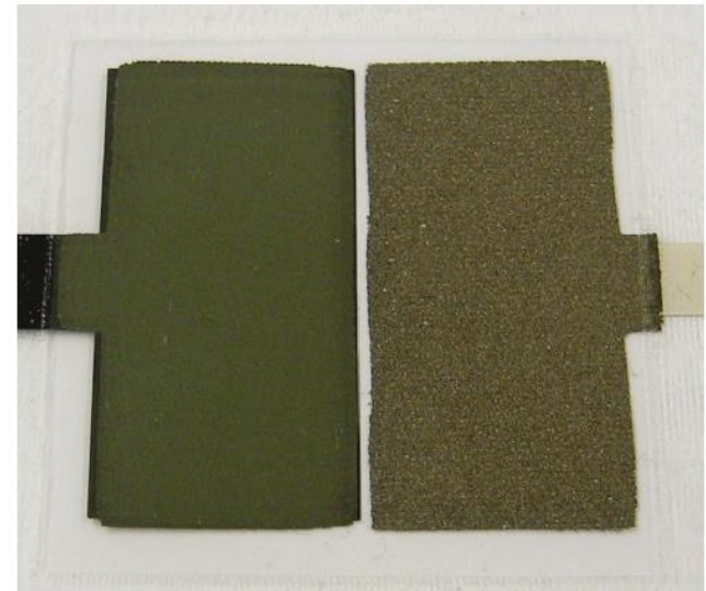
Figure 8.13 Example of a printed co-planar nickel/metal hydride battery. The device was fabricated in HdM, Stuttgart, Germany.
