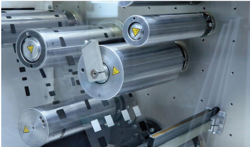
Printing Zinc \text{MnO}_2 batteries (from CENTI, Portugal)
